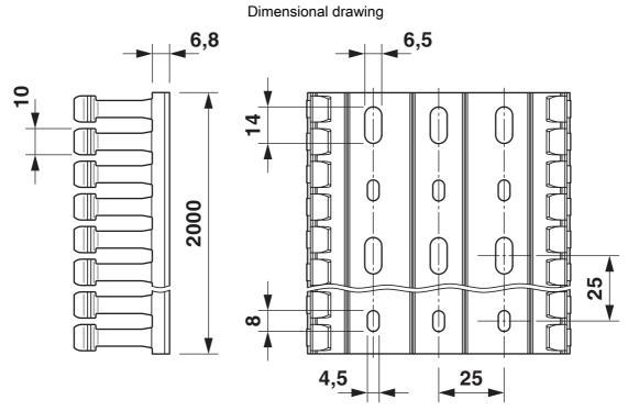
Base perforation according to DIN EN 50085
