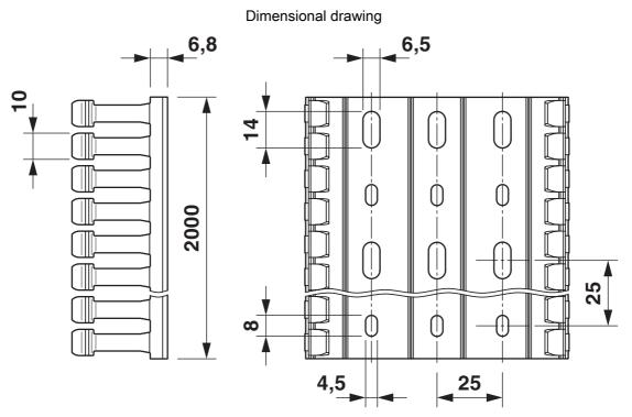
Base perforation according to DIN EN 50085
